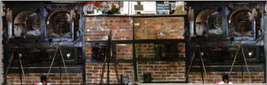
Document 241: Composite photograph based on the TOPF double-muffle cremation furnace at Gusen Camp illustrating the structure of the Topf eight-muffle furnace.
