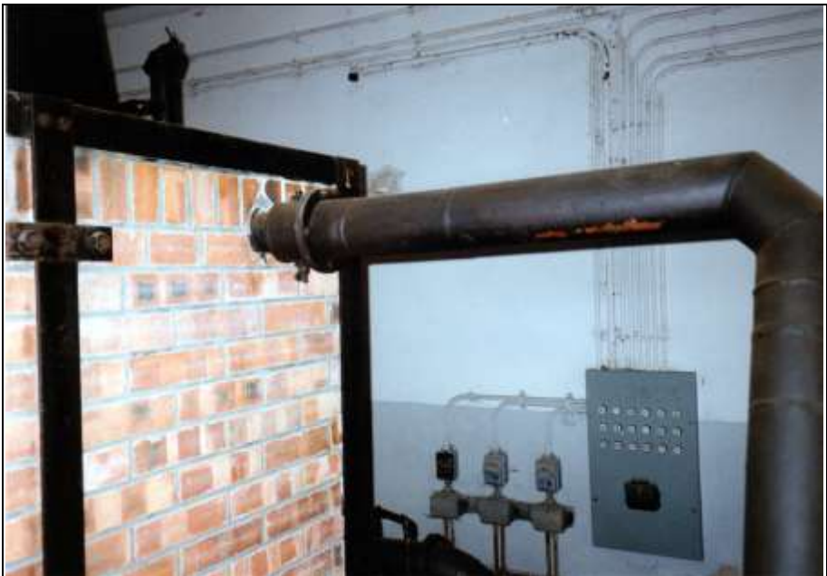
Photograph 192: Blower tube connected to the furnace fueled with either naphtha or coke. At the tube's end, close to the furnace's wall, is a valve for regulating the air flow.
