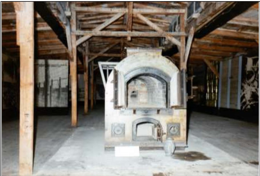
Photograph 319: as above; top: the muffle door; bottom center: ash-chamber door; bottom left and right: combustion-air inlets.
