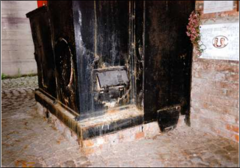
Photograph 34: The rear of the furnace with chimney (left-hand side) with an access door to a pilot flame at the chimney's base. The circular sheet metal welded to the chimney's base closes the original opening for a forced-draft blower.
