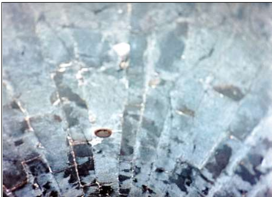
Photograph 60: Vaulted ceiling of the left-hand muffle; outlets of pipes connected to the blower.
