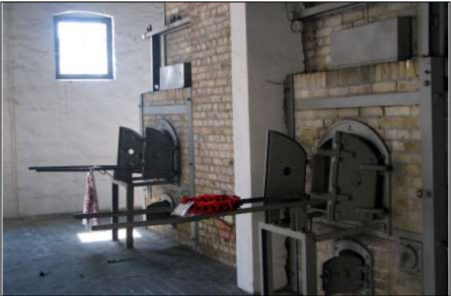
Photograph 338: KORI coke- and naphtha-fired cremation furnace at Ravensbrück Concentration Camp. Source: http://mmlorusso.blogspot.com/2011/03/his-will-is-our-hiding-place-cont.html .
