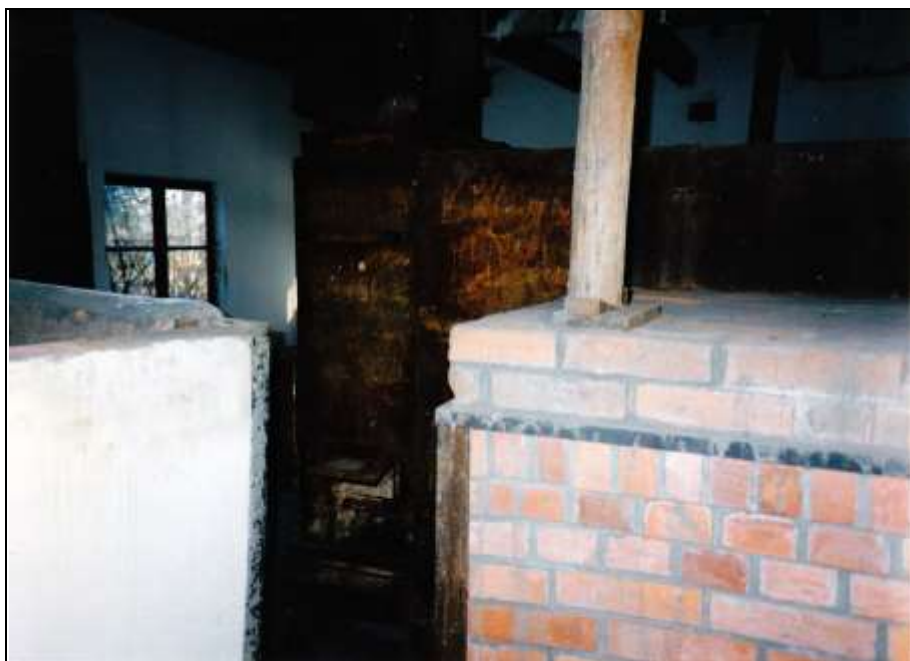
Photograph 50: Left-hand side of the furnace; background: open service door for the pilot flame at the chimney's base.
