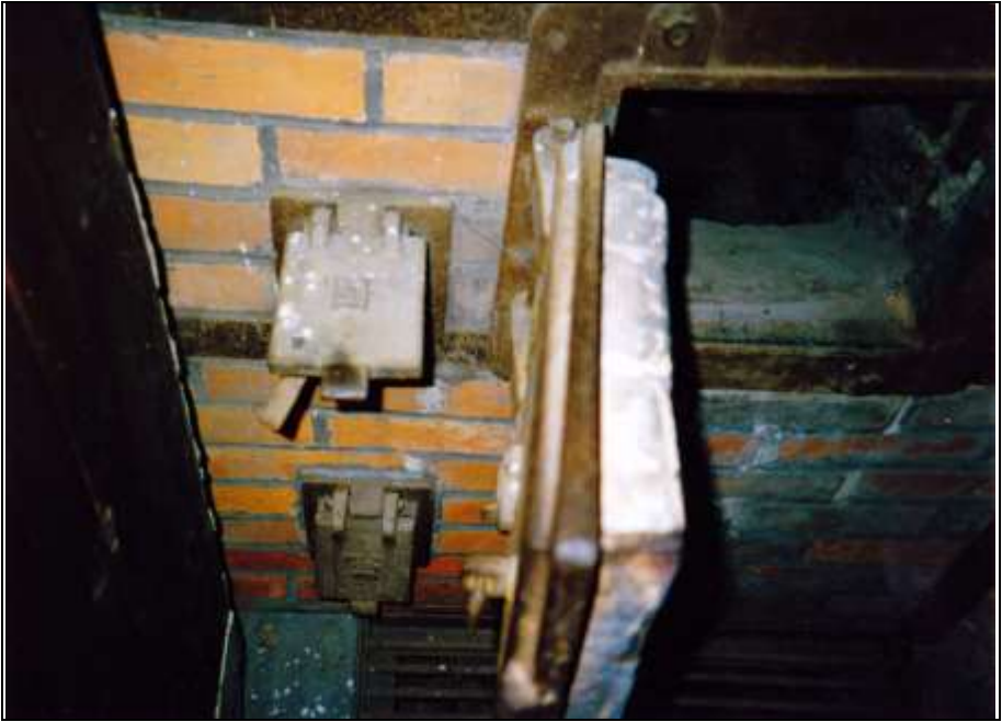
Photograph 39: Left-hand gasifier: large coke-loading door (right), small doors for the primary air to the hearth (bottom) and the primary air to the gasifier (top).
