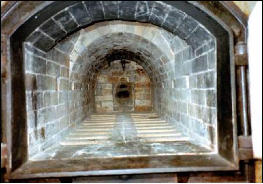
Photograph 320: Inside of the muffle. Bottom: the refractory grate; on the back wall: the main burner's nozzle; on the side walls: openings of the combustion-air-supply channels.
