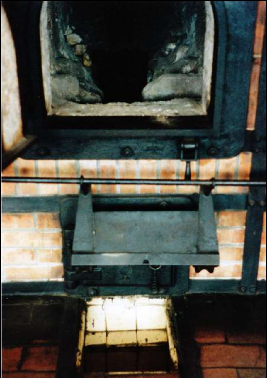
Photograph 178: as above, front view, central muffle. The lowered movable roller device. The device is threaded through the mounting bar, can pivot vertically and move horizontally.
