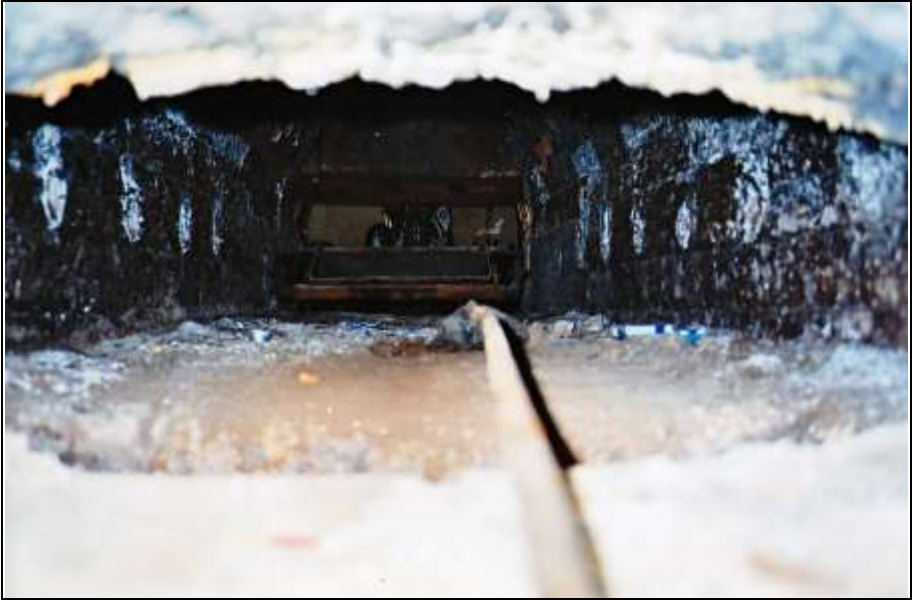
Photograph 353: as above, with the introduction cart pulled out. In the foreground, the shaft of the scraper to remove cremation remains.
